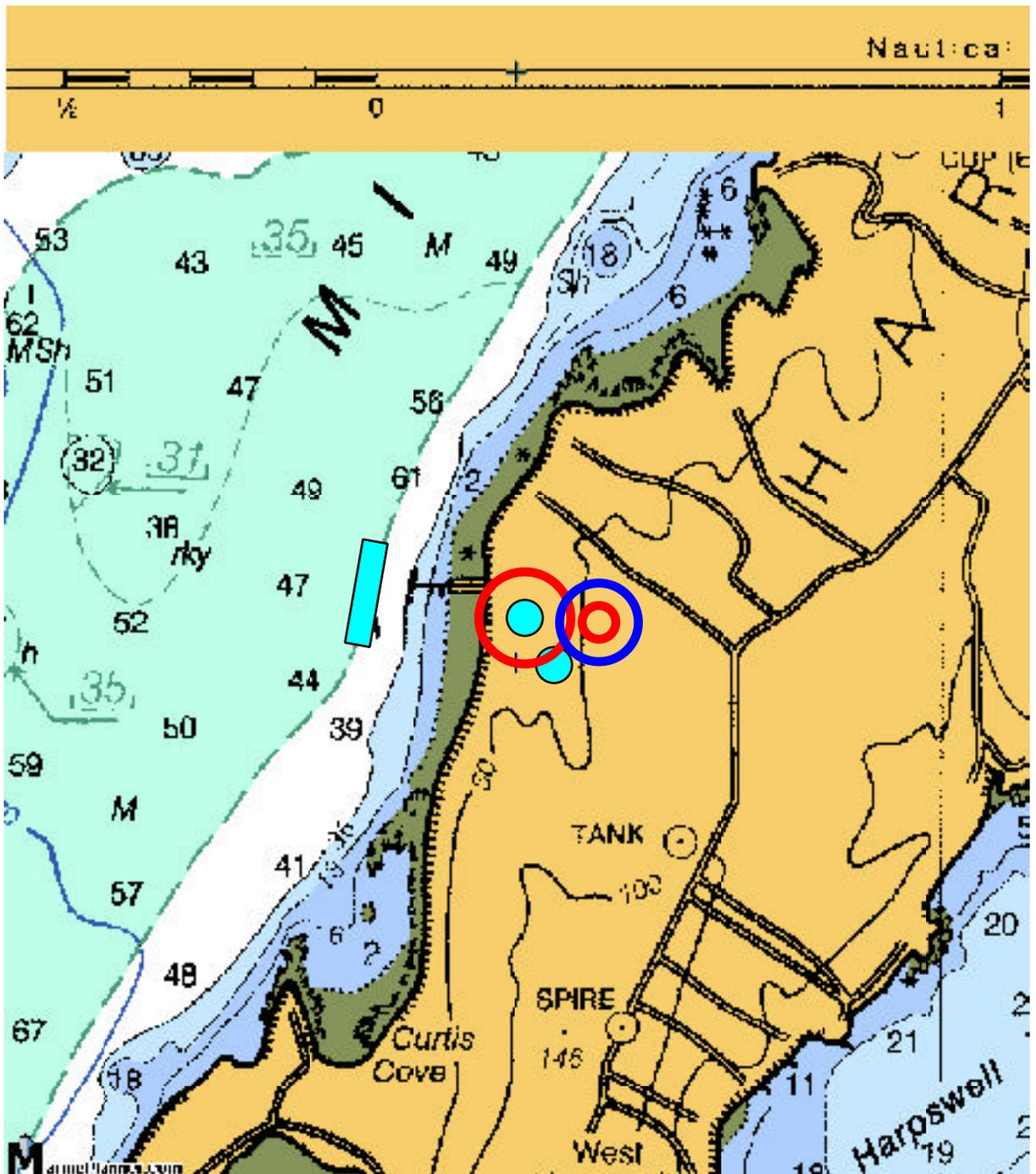
Figure 2: FERC-defined thermal radiation and flammability zones for the proposed Harpswell LNG terminal. Red circles are distances to radiation intensities of 5 kW/m<sup>2</sup> for a spill with fire; blue circle is the distance to the flammability limit for a spill without fire. Large red circle is for failure of primary tank containment; small red and blue circles are for transfer piping release.
