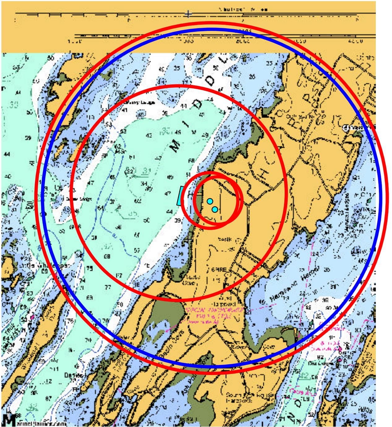
Figure 3: The non-FERC flammability and radiation distances of Table 2. Red circles are distances to radiation intensities of  $1.6 \text{ kW/m}^2$  for a spill with fire; blue circle is the distance to the flammability limit for a spill without fire. Largest red circle is for failure of secondary tank containment; next smaller red circles: tanker hold contents, primary tank, and transfer piping. Blue circle is loss of primary containment.
